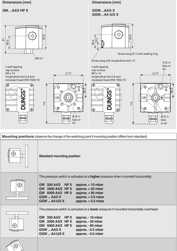
If mounted in intermediate mounting position, the pressure switch is activated at a max. higher or lower pressure compared to the set nominal value.
